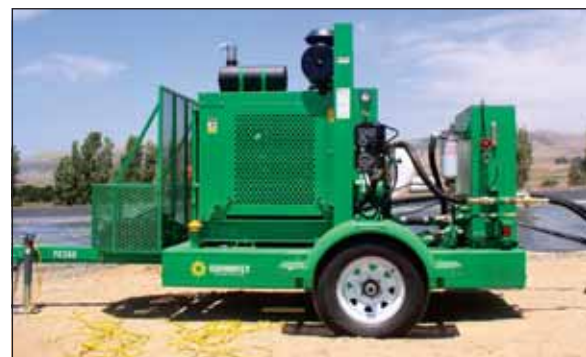
Gulf Atlantic ZU-100JT 100 HP Hydraulic Power Pack
