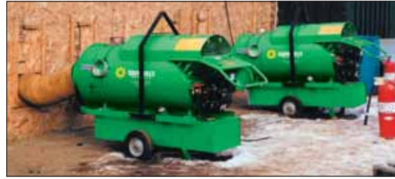
(2) ICE OHV 350 320,000 BTU Oil Indirect-Fired Shown heating a temporary construction building
