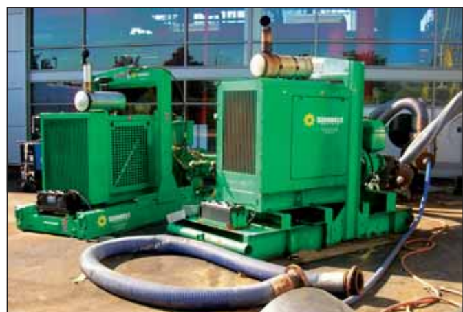
(2) Gorman-Rupp Diesel High Head Pumps
