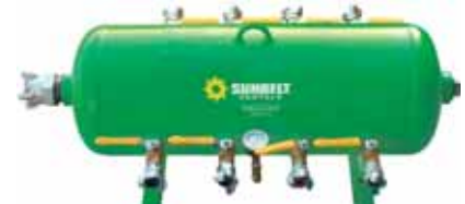
Tank-Type Air Manifold (8) ball valve controlled outlets 2" air inlet with 4-prong coupler on one end and flow-through plug on the other end allows using multiple units in tandem. Texas Pneumatic TX-2AMF
