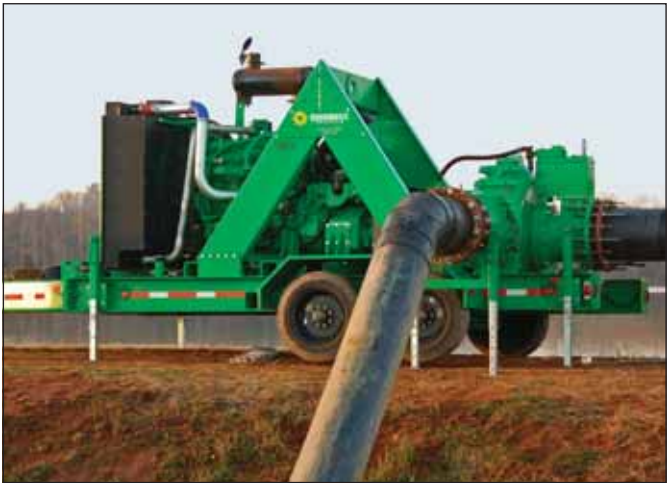
Premier 24" x 24" Diesel Trash Pump Working on an emergency dewatering project
